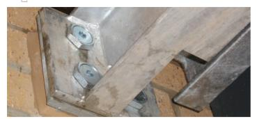
**BoxBolt** is a fully tested and approved blind connection solution for connecting to hollow section steel or where access is restricted to one side only. The **BoxBolt** is suitable for use with rectangular, square and even circular hollow sections. The **BoxBolt** features a hexagon head design to aid installation with a standard wrench. It allows it to be installed with our unique **BoxSok™** installation tool for when installation time needs to be kept to an absolute minimum.
