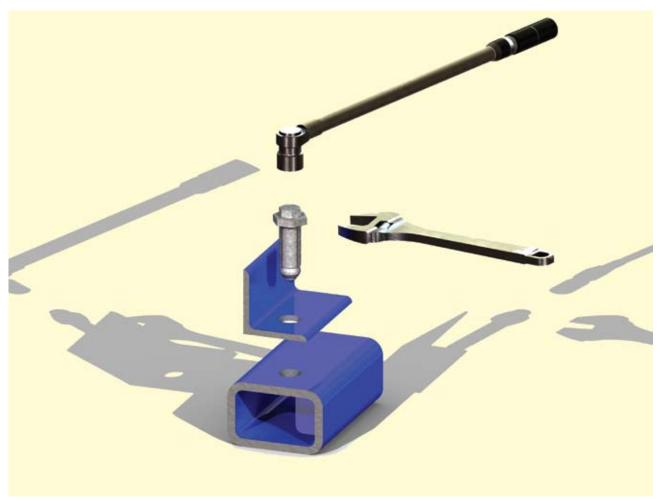
**STEP 1:** Align the holes in the bracket to be secured with the pre-drilled hole in the structural tube. Insert the BoxBolt through both pieces of steel until the underside of the shoulder is flush with the outside of the steel.
