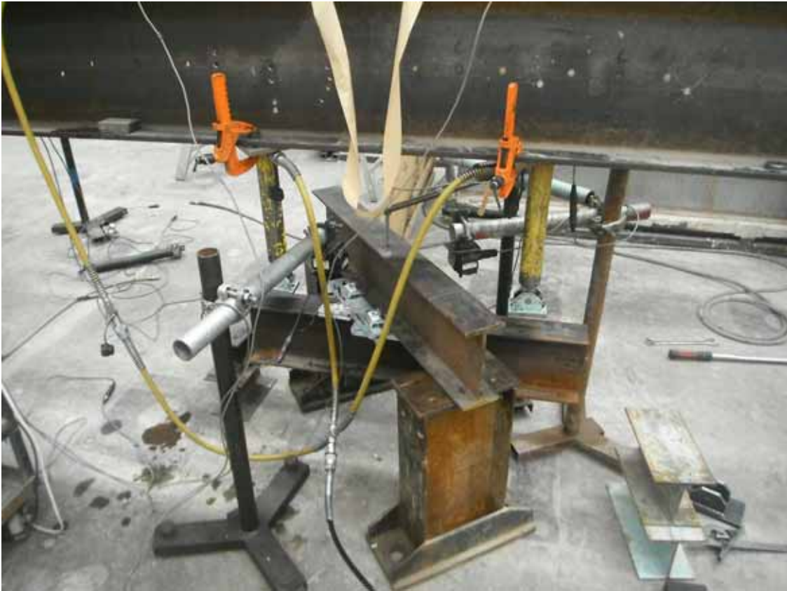
Plate 2 - General View of Tensile Test Arrangement for the Fast Fit BeamClamp System with a 45 Degree Configuration
