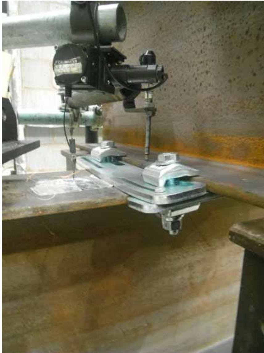
Plate 4 - Typical Failure of the Fast Fit BeamClamp System with a 90 Degree Configuration
