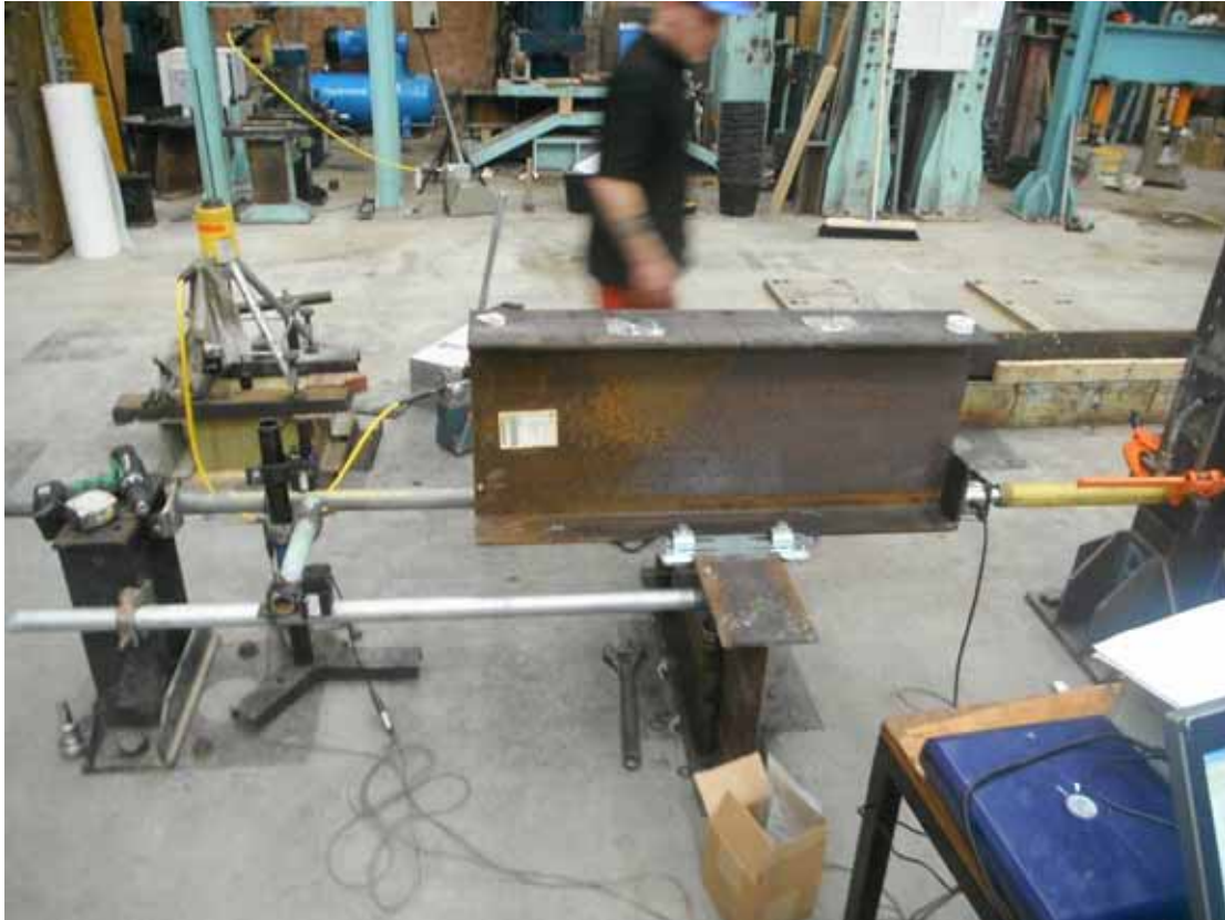
Plate 3 - General View of Frictional Test Arrangement for the Fast Fit BeamClamp System
