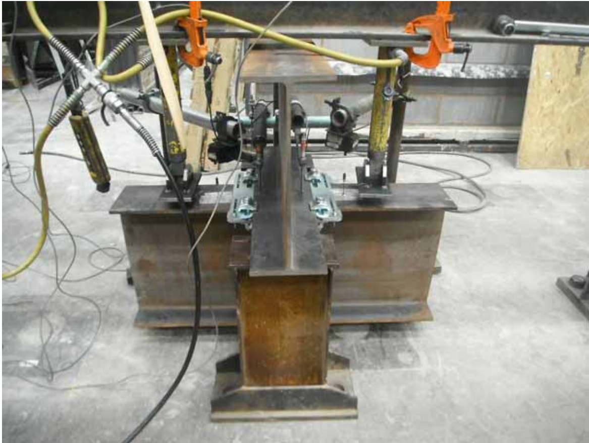
Plate 1 - General View of Tensile Test Arrangement for the Fast Fit BeamClamp System with a 90 Degree Configuration
