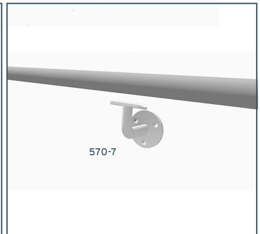
C) WALL MOUNT: The 570-7 is connected to the wall or wood posts using 1/4" screws or bolts. The 570-7 is attached to the railing with No. 12 self-drilling screws.
