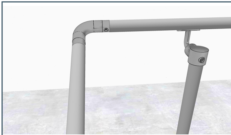
Supporting joints: All elbows and angles should be supported with a post no further than 18 inches from the join.
