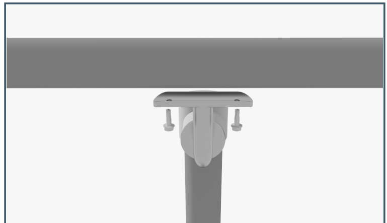
HANDRAIL BRACKET ATTACHMENT: Brackets attach to the handrail pipe with two No. 12 self drilling screws or pop rivets. Use high quality hardware for the best results.
