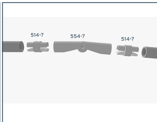
E) ADJUSTABLE ANGLES: In order to accomplish angles with a smooth surface, use the 554-7 and two 514-7. These are frequently used at the top and bottom of ramps and stairs.
